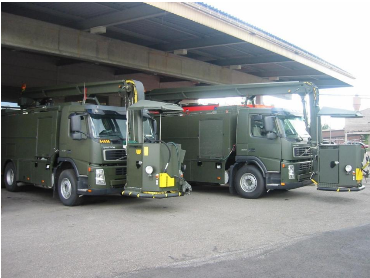
De-icing platform vehicle (DDP 45/23)
