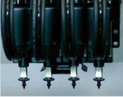
New lightweight full-servo head (Optional 4-axis 4-theta head)
